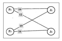
$\begin{array}{l} \mbox{Min cost } P_2 \rightarrow J_3 = 12 \\ \mbox{Delete } P_2 \mbox{ and } J_3 \end{array}$
